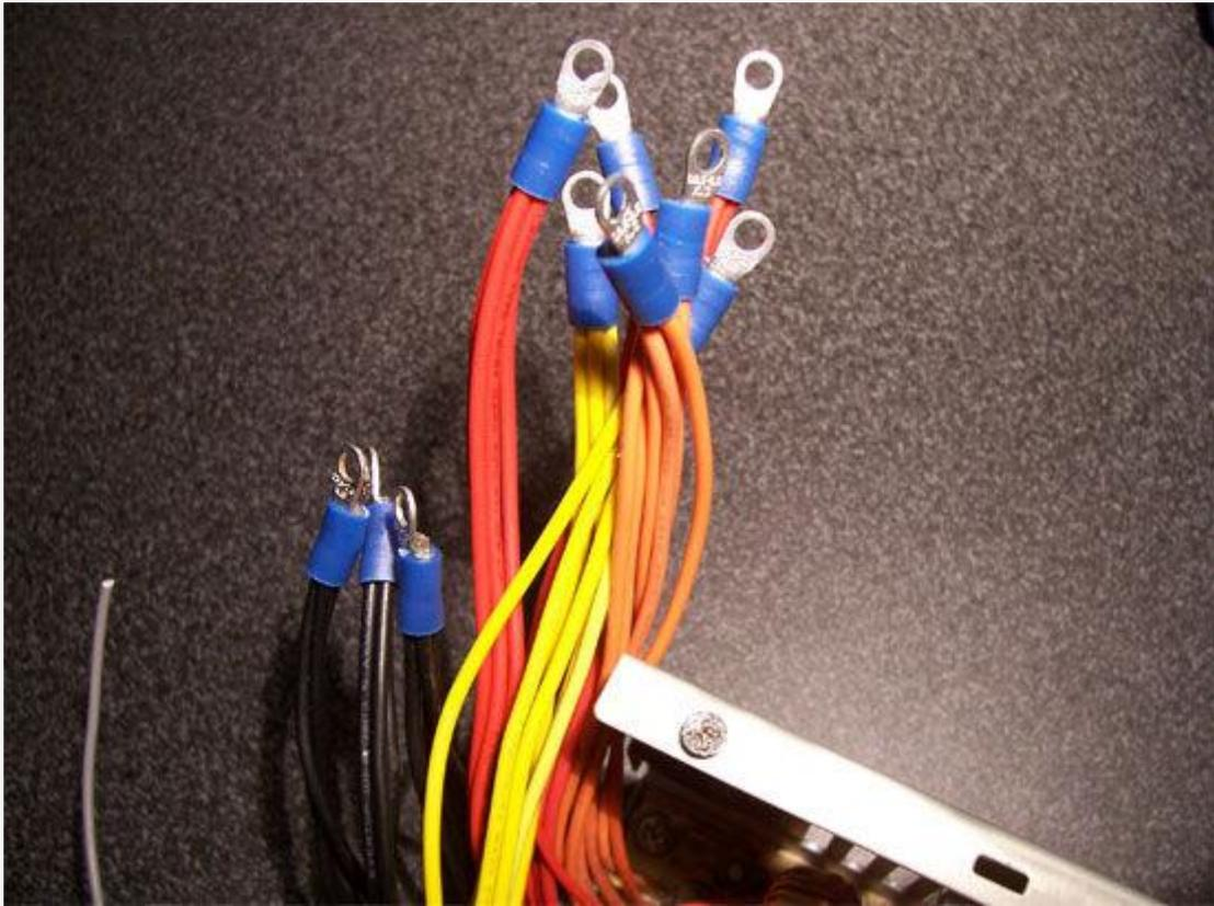
Group the 4 wire colors together and cut them to length to where you marked where the posts would go. Use the wire strippers to take off the insulation and stick about 3-4 wires into one tongue terminal. Then crimp them. The exact number of wires per voltage rail depends on the wattage of the PSU. Mine was a 400W and there are about 9 wires per rail. You need all these wires so that you can get all of the current rated for that rail.
