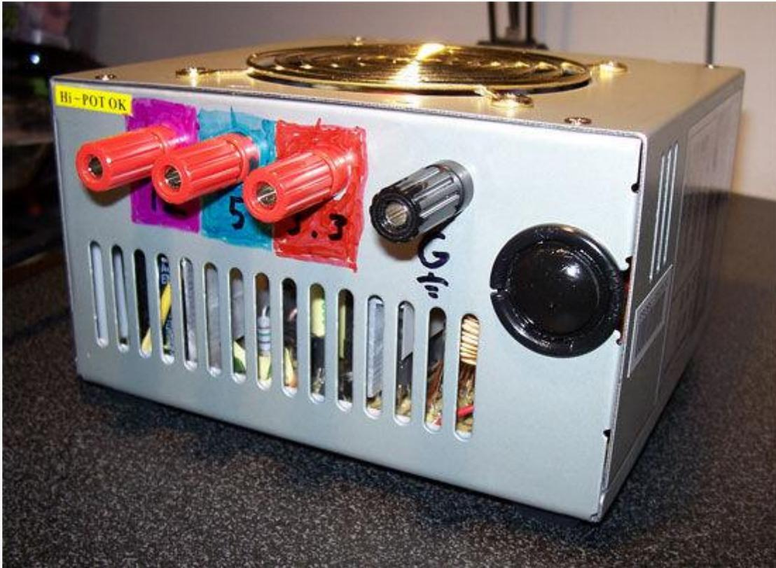
My 400 Watt power supply can deliver 23 Amps through the 12V rail, and 40 Amps through the 5V. That's very good for something that, aside from the initial cost of the PSU, cost about \$10.
